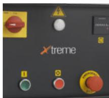
Low voltage (24V) control panel with star-delta system
